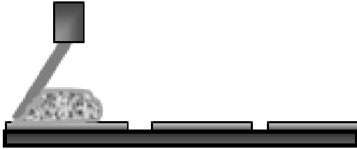
Figure 3a. Contact angle 60^{\circ} prior to print stroke
