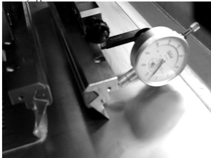
Figure 4. Blade holder set up for 0.007” thick blade. No pressure applied.
