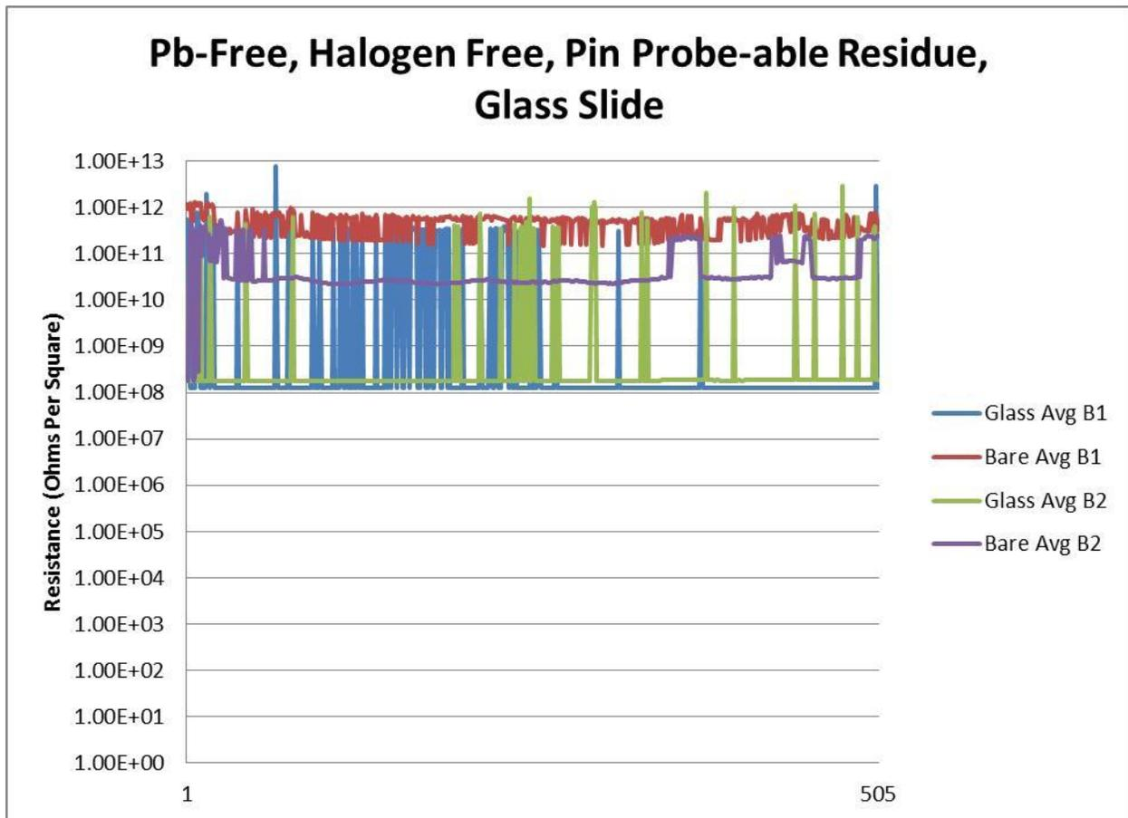
Both the bare patterns and the patterns covered with the glass slides produced passing SIR values. However, the patterns covered with the glass slides exhibit lower SIR performance.
