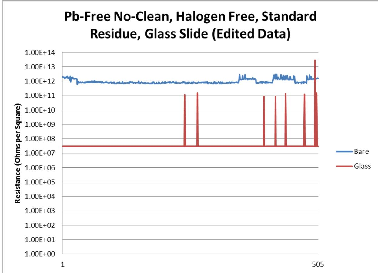
The bare patterns exhibit passing SIR values; whereas, the glass slide covered patterns exhibit lower and failing SIR values.
