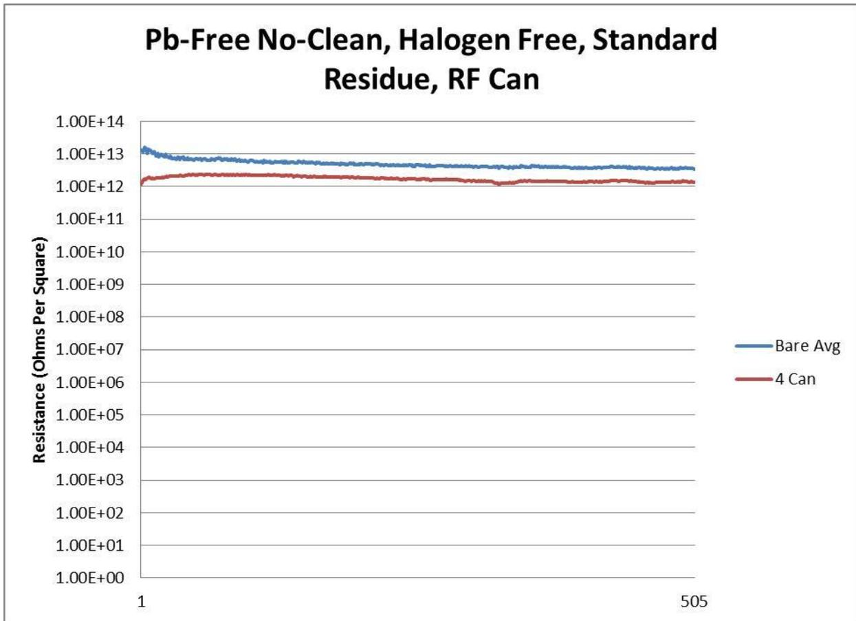
Both the bare patterns and the pattern covered with the RF shield produced passing SIR values. However, the pattern covered with the RF shield exhibits slightly lower SIR performance.
