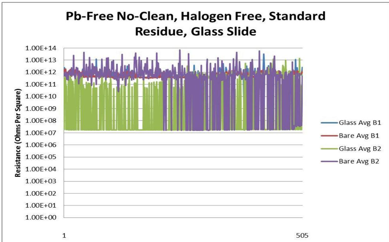
The author was not able to ascertain any meaningful trend from the data produced from these two boards. There seemed to be no rhyme or reason to it. Possible explanations for the aberrant data include condensation, improper wiring, loose connections, etc. Therefore, the author selected data sets that seemed to be in agreement with the typical SIR trend of bare and glass covered patterns. That data is in the following graph.
