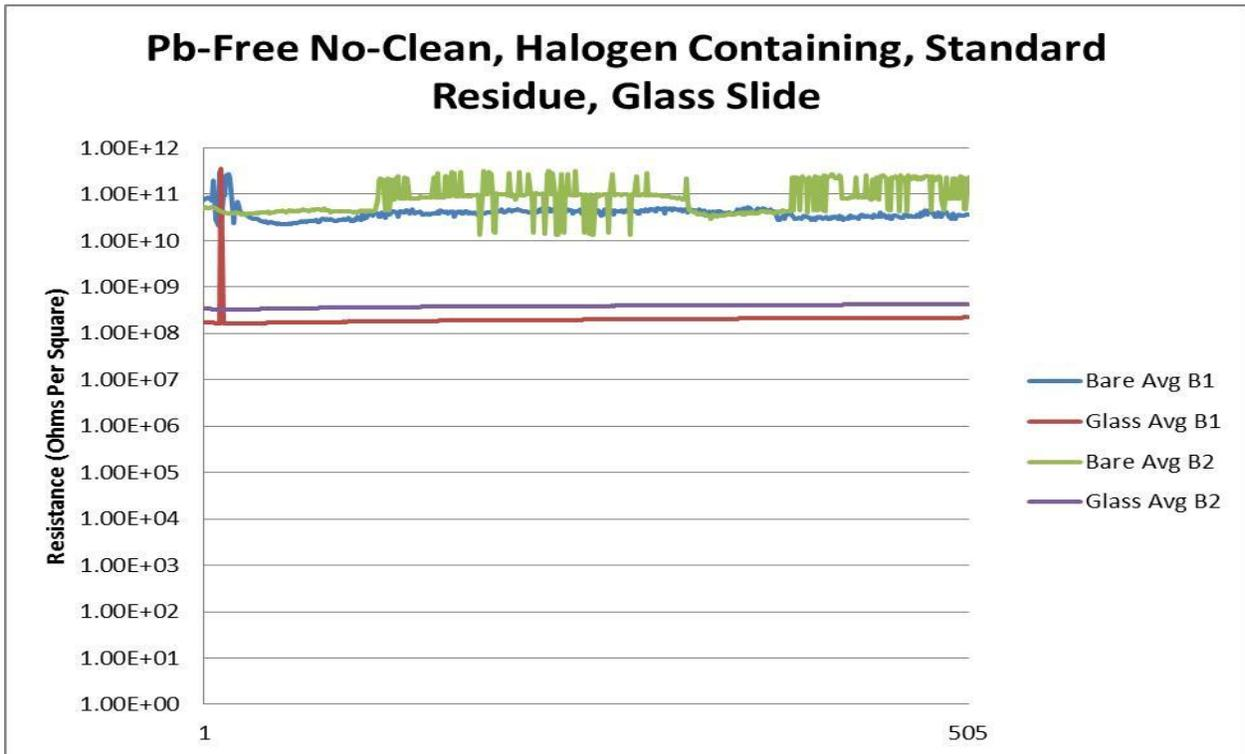
Both the bare patterns and the patterns covered with the glass slides produced passing SIR values. However, the patterns covered with the glass slides exhibit lower SIR performance.
