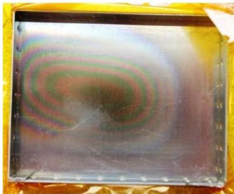
**Figure 12 - Discoloration of the RF Shield**
