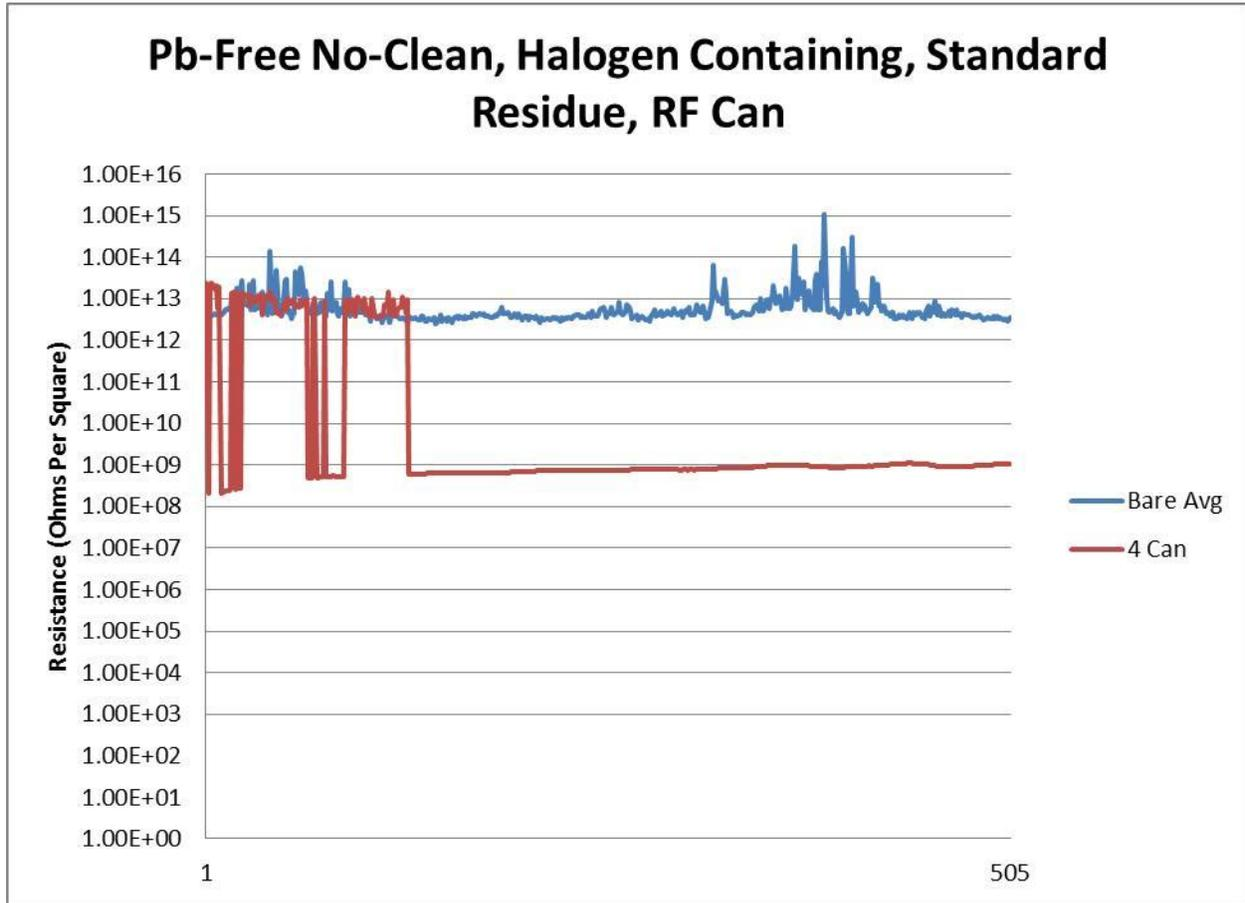
Both the bare patterns and the pattern covered with the RF shield produced passing SIR values. However, the pattern covered with the RF shield exhibits lower SIR performance.
