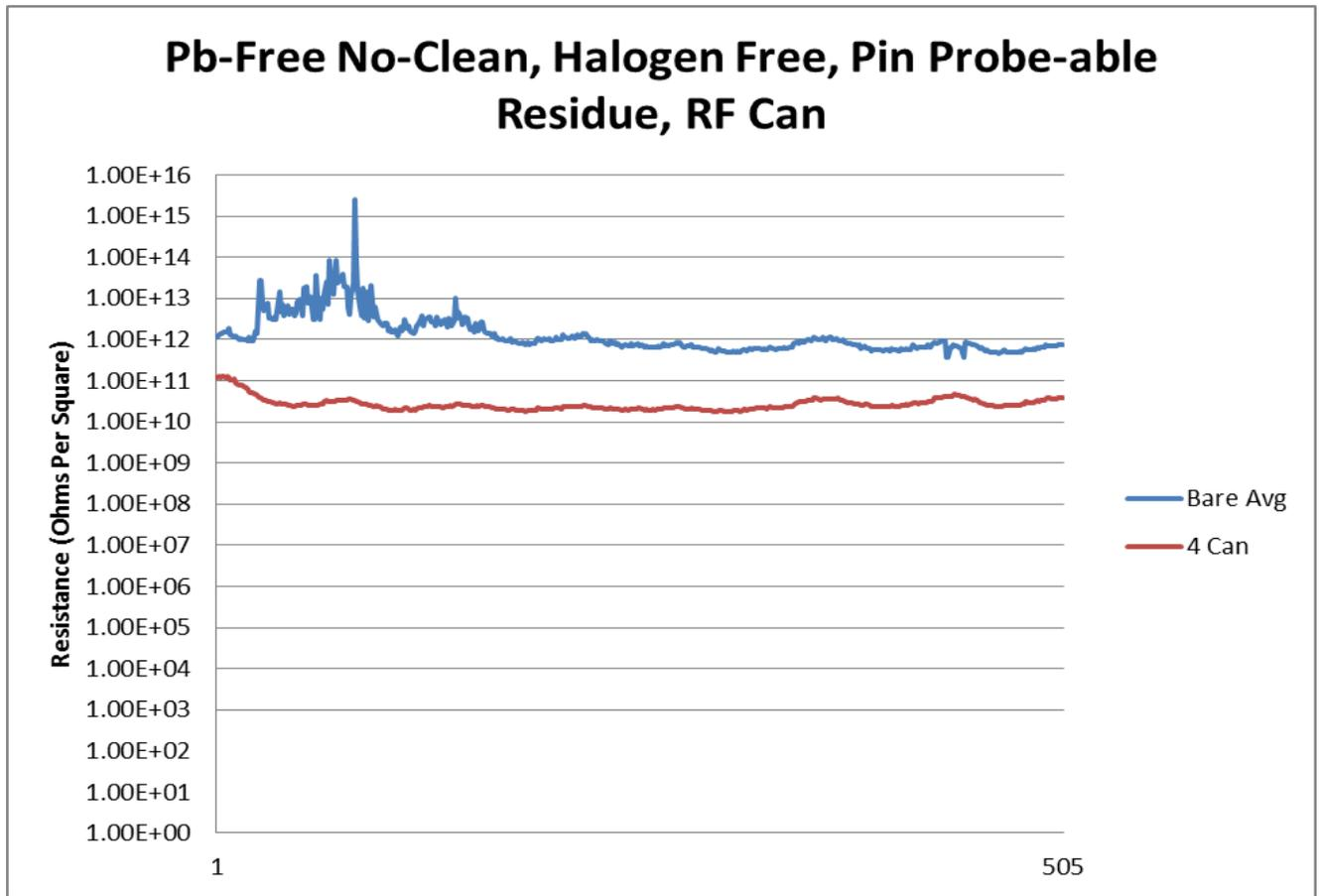
Both the bare patterns and the pattern covered with the RF shield produced passing SIR values. However, the pattern covered with the RF shield exhibits slightly lower SIR performance.
