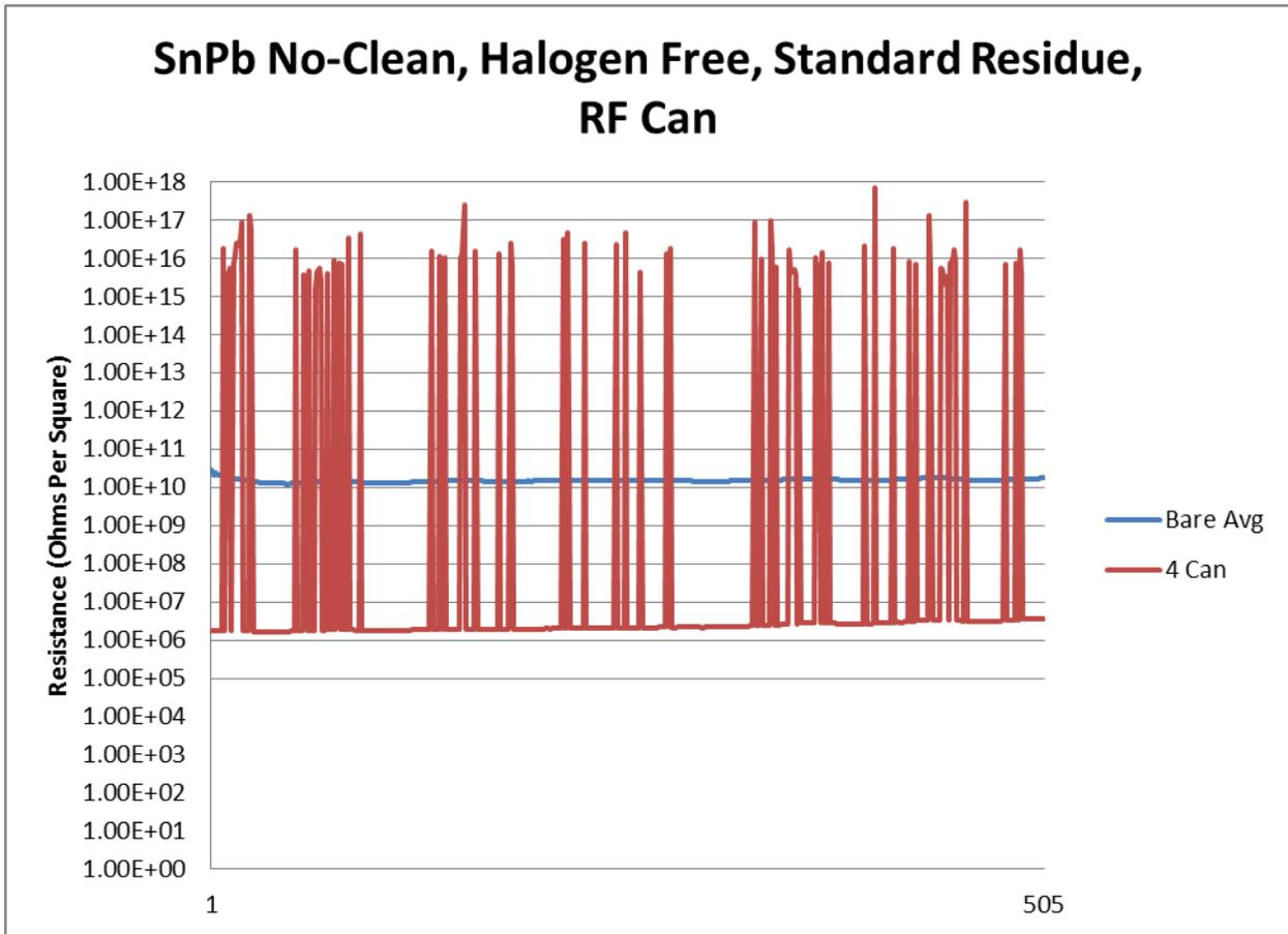
The bare patterns exhibit passing SIR values; whereas, the RF shield covered pattern is virtually shorted. (It is not possible to get readings less than 1.00E+6 because of a 1M $\Omega$  current limiting resistor in the circuit.)
