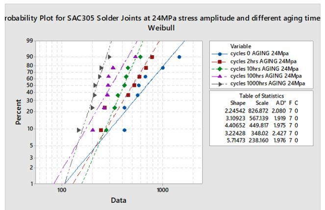
(c) Two-parameter Weibull distributions under 24 MPa stress amplitude and different aging times
