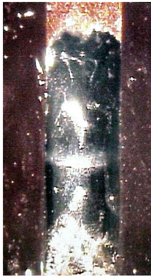
( Figure 9, using the dross elimination material, note improved wetting)
