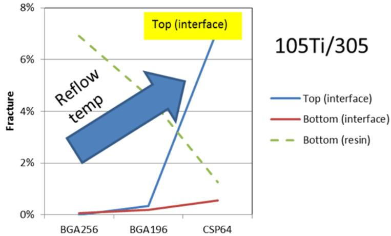
Figure 12 - Relation between reflow temperature and fracture site for 105Ti/305
