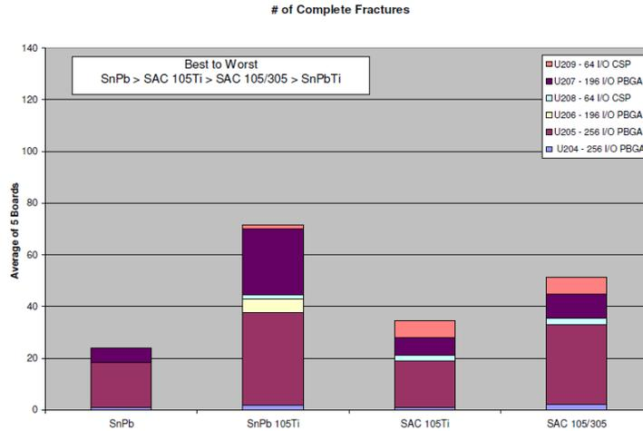
**Figure 4 - Results of dye and pry test with complete fractures. Data presented is average of 5 boards.**
