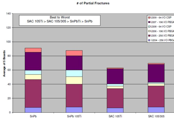
**Figure 5 - Results of dye and pry test with partial fractures. Data presented is average of 5 boards.**
