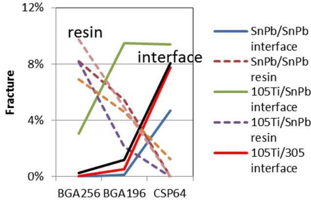
Figure 9 - Effect of package type on fracture
