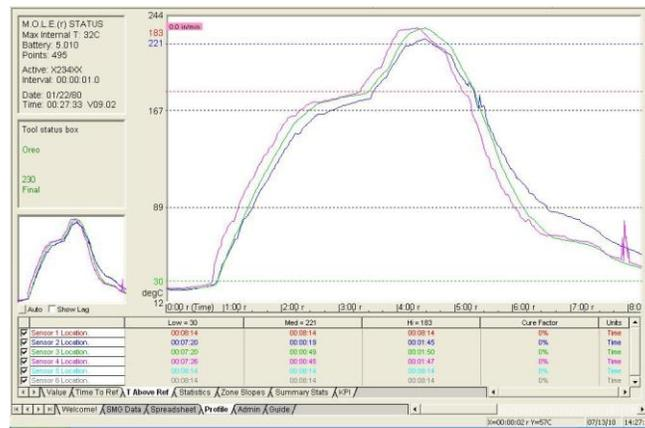
Figure 3 - Reflow profile 2, with peak temperature 230+3 °C, and 60±10 seconds above 183 °C.
