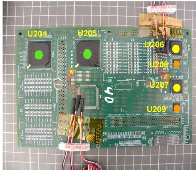
**Figure 1 - Test vehicle layout, with two BGA256 (U204, U205, in green), two BGA196 (U206, U207, in yellow), and two CSP64 (U208, U209, in orange) located on the board.**
