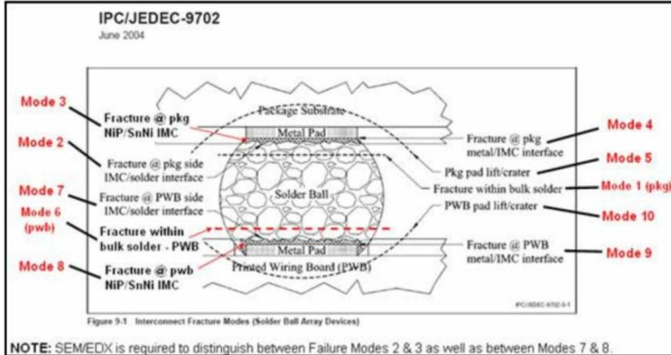
Figure 6 - Interconnect fracture modes (solder ball array device) IPC/JEDEC-9702.
