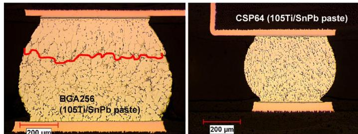
Figure 8 - Microstructure of BGA256 and CSP64 (SAC105Ti/SnPb paste) with the same profile setting.
