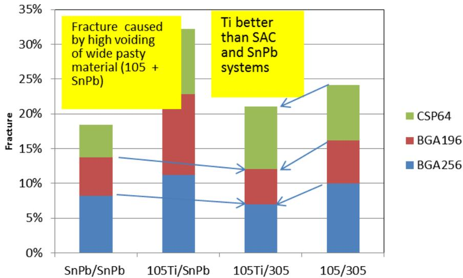
**Figure 10 - Effect of alloy combination on fracture**
