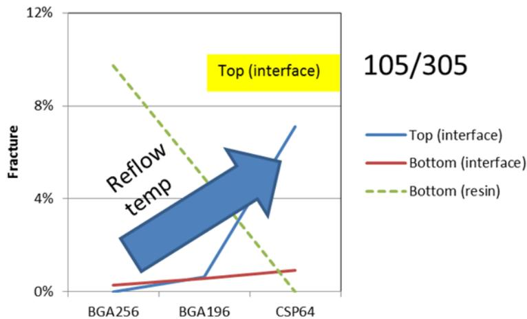
Figure 13 - Relation between reflow temperature and fracture site for 105/305
