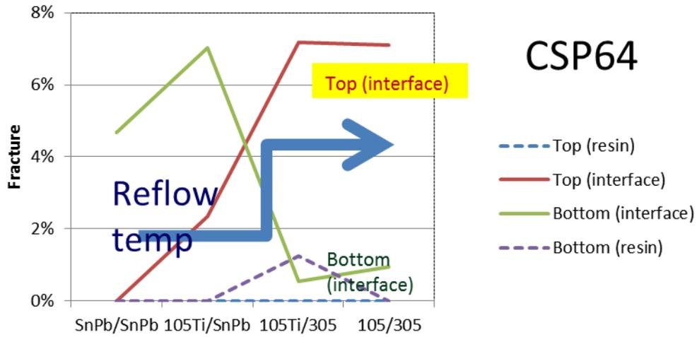
Figure 11 - Relation between reflow temperature and fracture site
