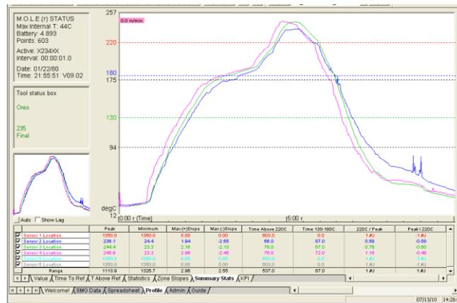
Figure 2 - Reflow profile 1, with peak temperature 235+3 °C, and 90±10 seconds above 217 °C.
