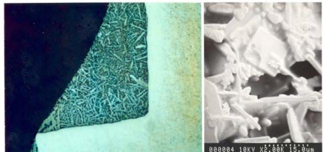
Figure 1: Gold-Tin IMC Images- Optical (left), SEM (right)
