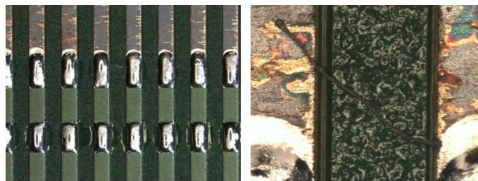
Figure 18 – Fiber assisted creep corrosion
