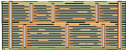
28 Layers – Two cores connected with PTH
