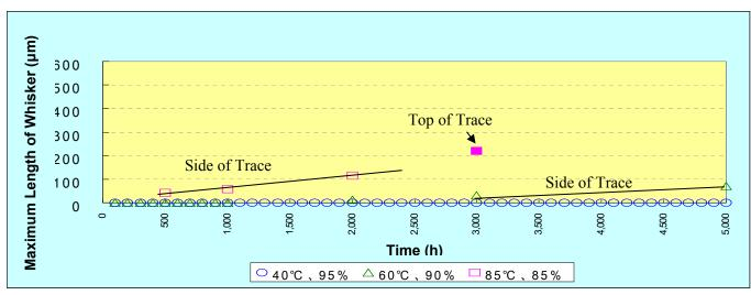
Figure 7. Maximum whisker length as a function of environment and time
