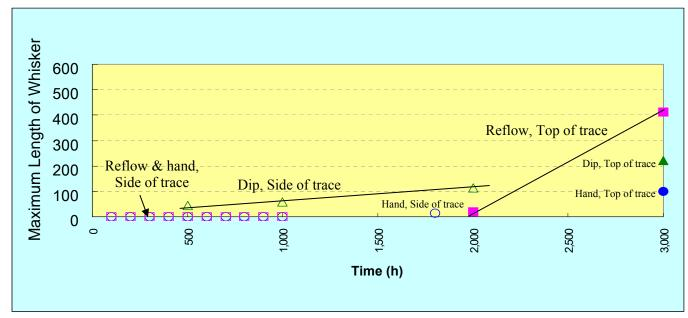
Figure 8. Maximum whisker length as a function of time at 85C/85%RH and soldering method
