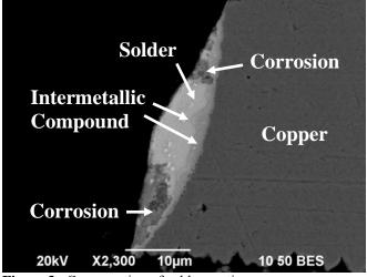
Figure 3. Cross-section of solder coating
