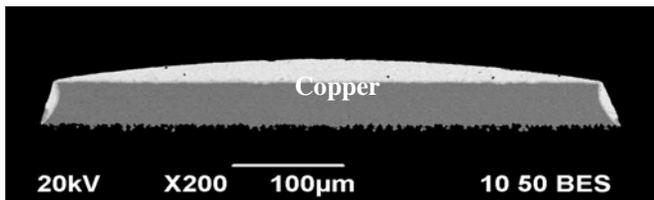
**Figure 2.** Cross-section of typical soldered trace
