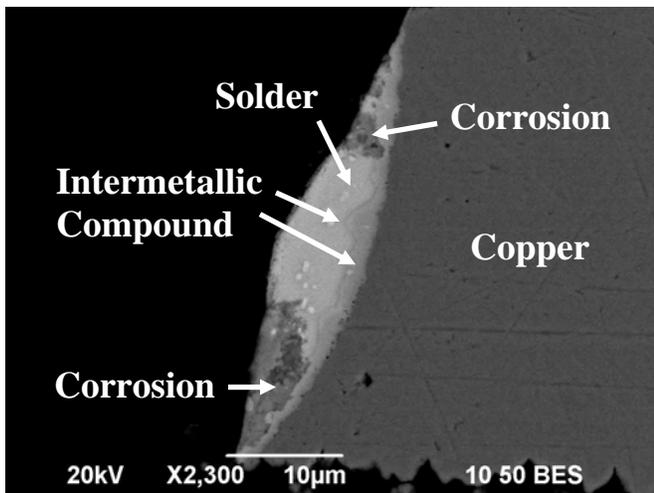
**Figure 3.** Cross-section of solder coating
