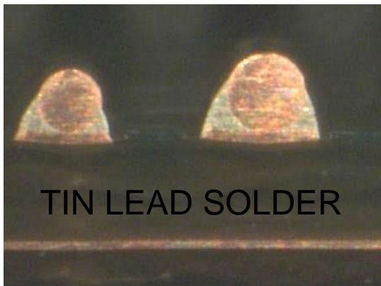
Figure 12: Solder cross section (Supplier 1)
