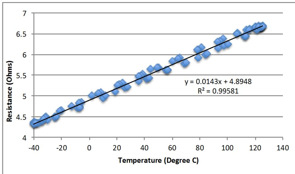
Figure 10. Resistance is a function of temperature
