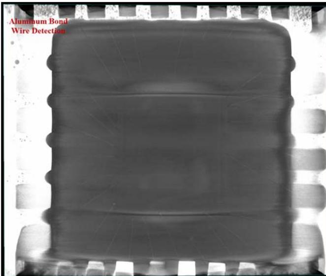
**Figure 6.** CT Image Showing Aluminum Bond Wires Inside a Package Utilizing the Black and White Histogram
