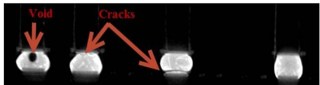
Figure 4. CT Slice Showing a Void and Cracks on BGAs with Enough Sensitivity to also show the vias and pads
