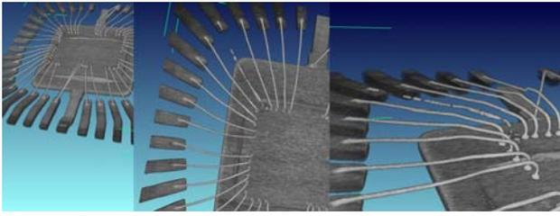
**Figure 5.** CT Scan Done in Under One Minute Showing a Failure on one of the Bond Wires
