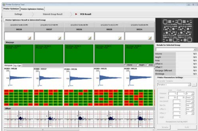
Figure 4: Automatic print process data analysis by SPI machine with feedback to printer
