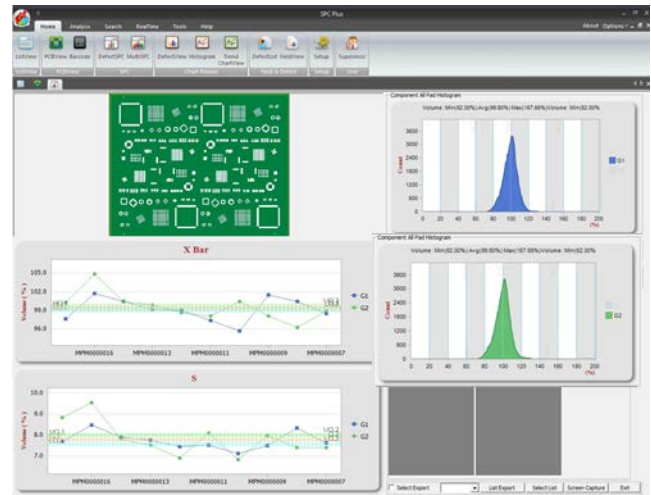
Figure 5: Advanced APC test results comparing human (blue) and software (green) printer optimization
