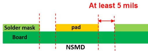
Figure 7 - The design of test coupons
