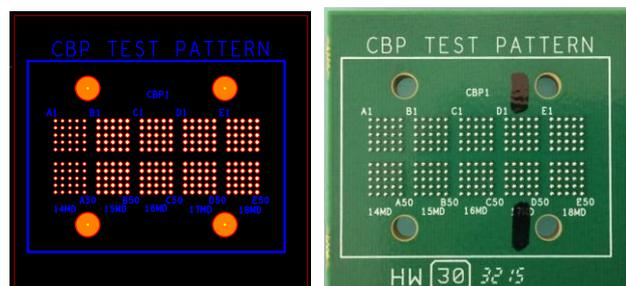
Figure 6 – Cold Ball Pull Coupon Design
