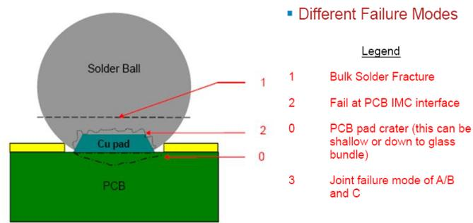
**Figure 9- The typical failure mode during CBP test**
