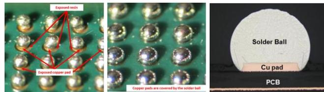
(a) Reject (b) Accept (c) Cross-section joint
