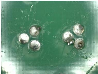
Figure 7: Wave Flux D (ActDry) Before Cleaning
