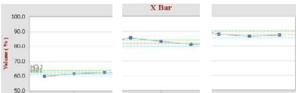
Figure 15. Percental volume transfer of a 0201 aperture for laser cut (left), laser cut & electro polished (middle) and PLASMA coated (right).
