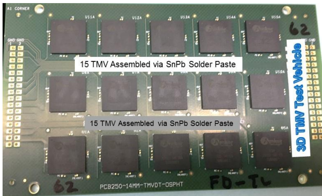
Figure 4. Fifteen 3D TMV™ daisy-chain package assembly with tin-lead solder either at package or PCB level.
