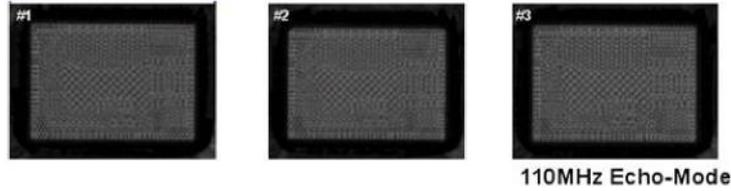
Fig. 22. Underfill void inspected by SAT.
