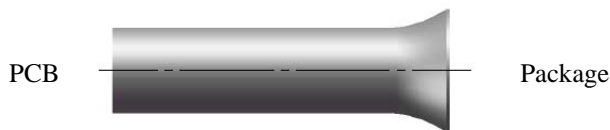
Figure 1. Pb90/Sn10 solder column shown with eutectic Sn63/Pb37 fillet.
