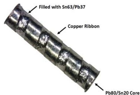
Figure 3. Pb80/Sn20 copper wrapped solder column without fillet (shown after coating with Sn63/Pb37)
