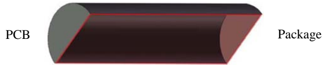
Figure 7. Sectional drawing of electroplated copper column over high melting temperature Pb90/Sn10 solder wire.
