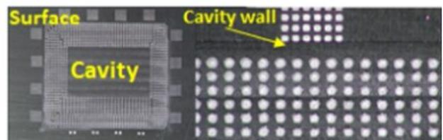
Figure 22. Print on cavity fixture
