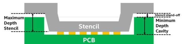
**Figure 9.** Illustration of PCB and stencil tolerance impacting stencil stand-off
