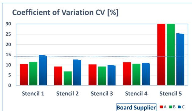
Figure 20. Board Supplier impact on print
