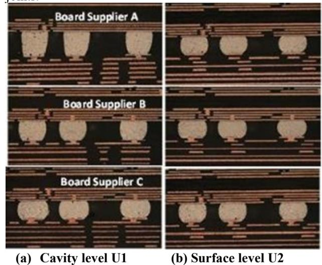
**Figure 30.** Comparison of BGA Solder Joints' Cross Section
