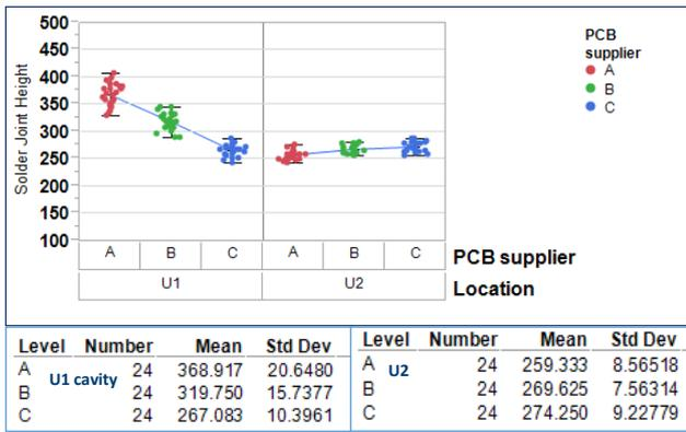
Figure 31. Solder joints height
