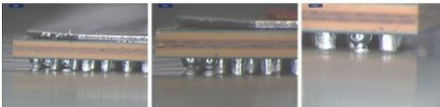
**Figure 28.** BGA Head on Pillow Defect
