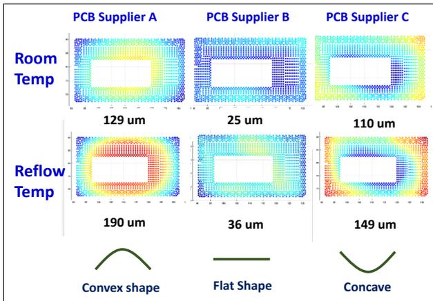
Figure 32. Warpage Shape and Magnitude for Boards from Three Different Suppliers
