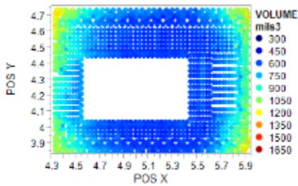
Figure 19. Paste volume distribution (welded stencil)
