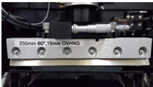
Figure 17. Slit Squeegee with a lateral adjustment head
