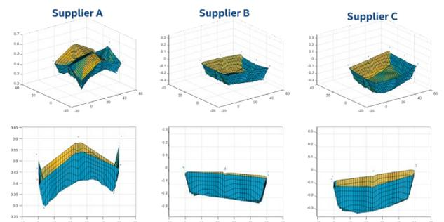
**Figure 10.** Cavity shape comparison for three PCB suppliers (at room temperature)
