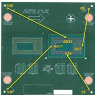
**Figure 11.** Approximate location of cavity registration measurement points and their associated labels
