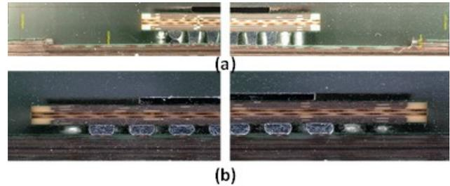
**Figure 29.** (a) Cross section U1 corners in the Cavity; (b) Cross section U2 corners on Board Surface
