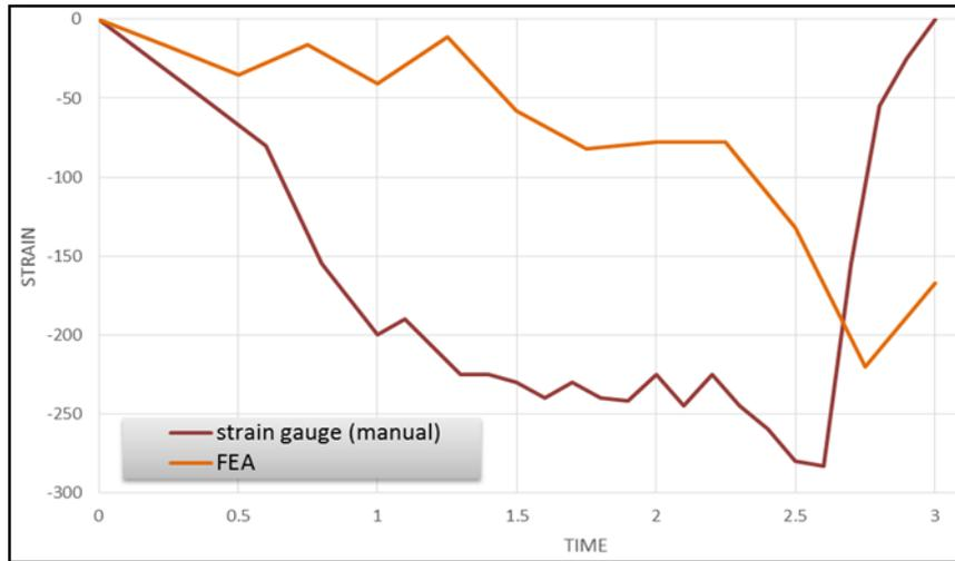
Figure 7. Max. Strain Graph (comparison for manual process)
