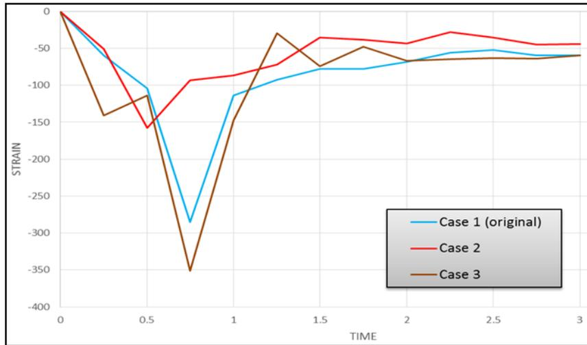
Figure 11. Max. Strain Graph (BGA location change)
