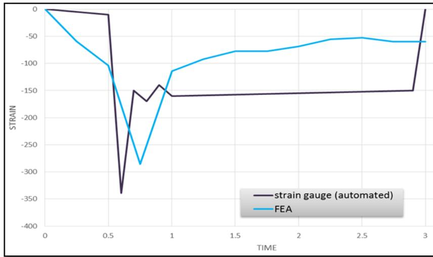
Figure 9. Max. Strain Graph (comparison for automated process)
