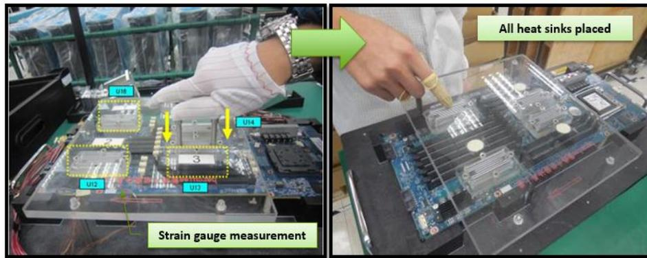
**Figure 1. Strain gauge on manual assembly set-up**
