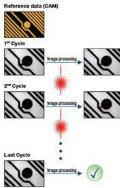
**Figure 2 – Rework Process**
