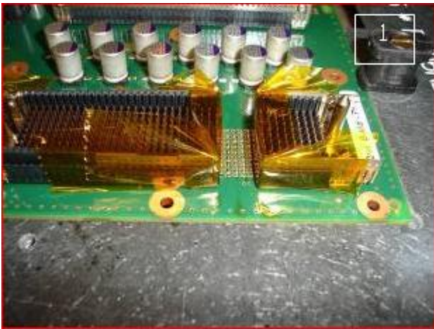
Figure 12: Kapton tape used to protect adjacent wafers during site dress
