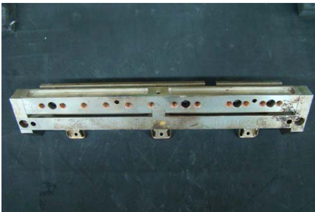
Figure 2: Fixture to apply uniform load across the connector
