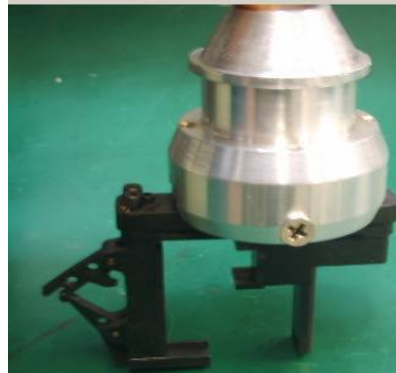
Figure 11: Rework nozzle for right angle receptacle
