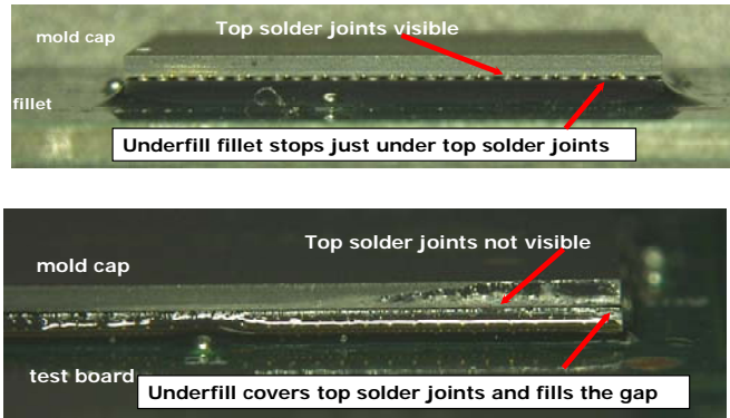
Figure 14: Cross sections of underfill coverage.
