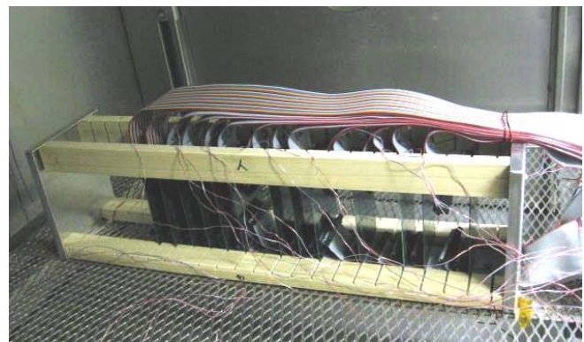
Figure 8: Rack of Package on Package Test Vehicles in ATC Chamber
