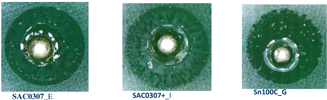
Figure 11 – Solder Ball Test Results_ Many Alternative Alloy Solder Pastes Resulted in Excessive Solder Balls
