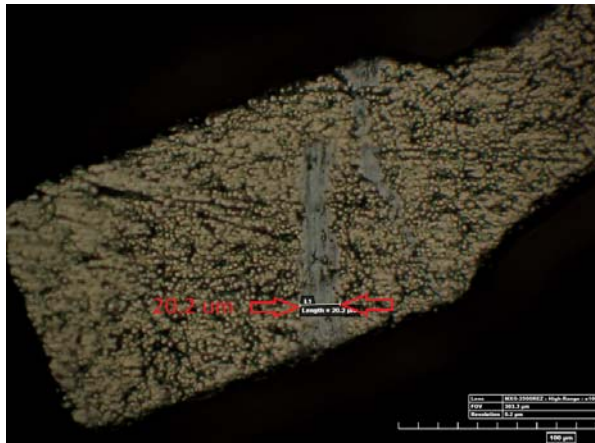
Figure 9 – Scratch Observed on Individually Defined Wire Bonding Pad on Rejected PCB
