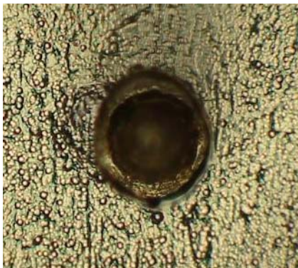
Figure 16 Wire Bond Made on Nodule
