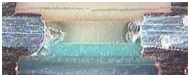
Figure 19. SJEM Dip2 cross section on the third row of package edge
