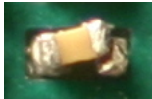
Figure 3. Skewed 01005 Component due to Inaccurate Placement
