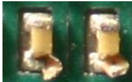
Figure 2. 01005 Termination Damage due to Excessive Force Applied during Placement
