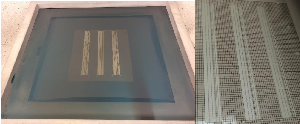
Figure 6 Test vehicle screen (left) and printed (right)
