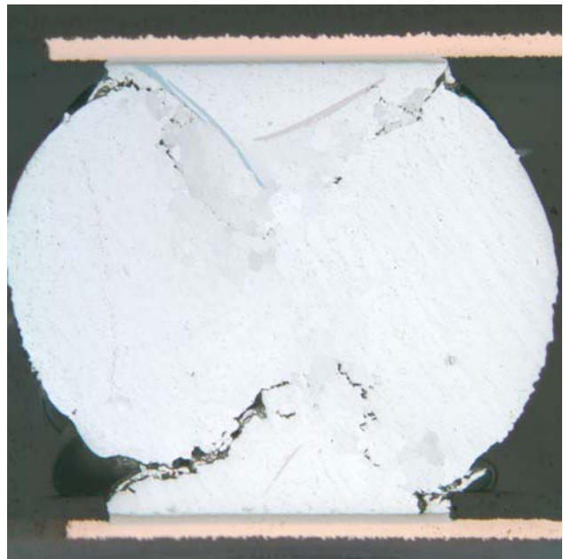
Figure 15. Thermal cycling cracks on top part combination B with underfill C.
