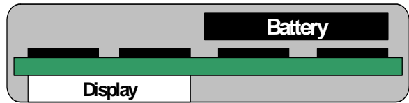
Figure 8. Basic structure of the cell phone used for the drop-testing.
