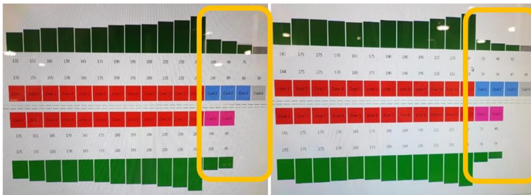
Figure 8 – Oven Cool Down Zones, Left -1.8°C/second, Right -3.4°C/second
