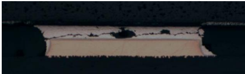
Figure 3 – Complete Crack Example, Outer Corner Locations
