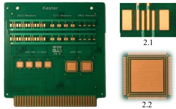
Figure 2. Custom-designed SIR board under Passives/QFNs
