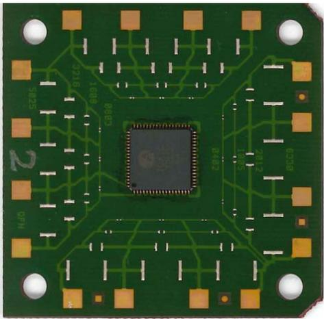
Figure 5. Test PCB for Thermal Cycle Test Evaluation (50x50mm)
