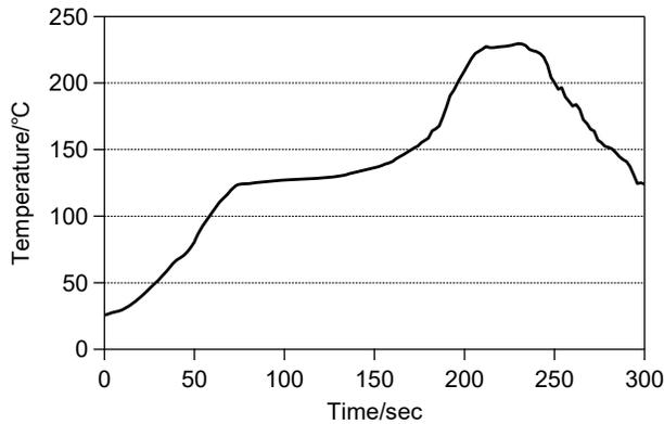
Figure 4. Reflow Profile (Air Atmosphere)
