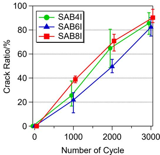
**Figure 9.** Crack Occurrence Transition on the Solder Joints of Test Solder Alloy and QFN/BTC
