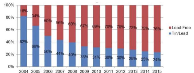
Figure 1. Solder paste delivery ratio, leaded and lead-free [1]
