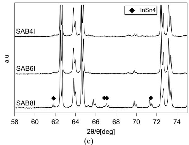
**Figure 8.** XRD Patterns for Each Solder Alloys (a) Overall View, (b) Expanded Micro-peaks at  $20\sim 40^\circ$  and (c) Expanded Micro-peaks at  $60\sim 75^\circ$
