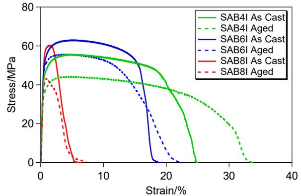
Figure 6. Stress-Strain Curve from Micro-dumbbell Pull Test
