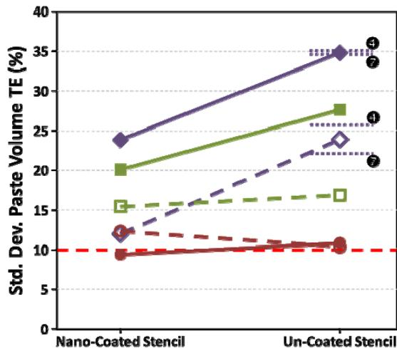
**Figure 14. M0201 Paste Volume Standard Deviations** (same legend applies from Figure 13)
