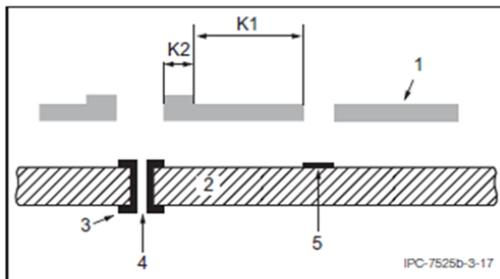
Figure 3-17 Overprint With Step (Squeegee Side)
