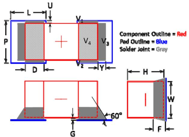
Figure 4. Minimum Solder Volume Termination Model
