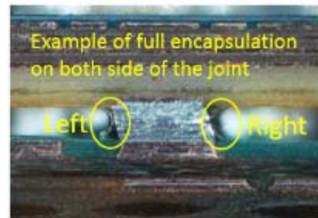
Figure 27. Pre-Temp Cycle, cross section location on two package location. Line1 = Edge coverage; Line15 = Closer to package die shadow region
