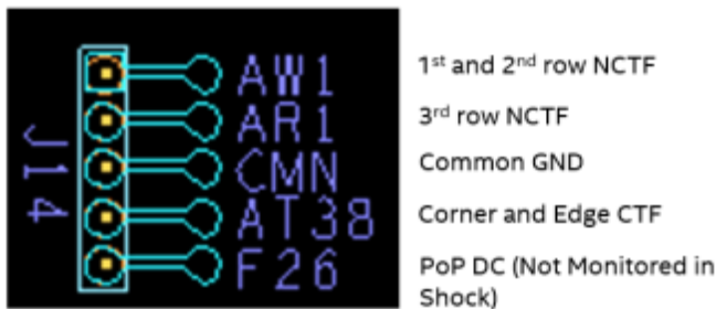
Figure 13. Daisy chain net designators for Shock and Temp cycle coverage. NCTF = Non critical to function; GND = Ground; CTF = Critical to function
