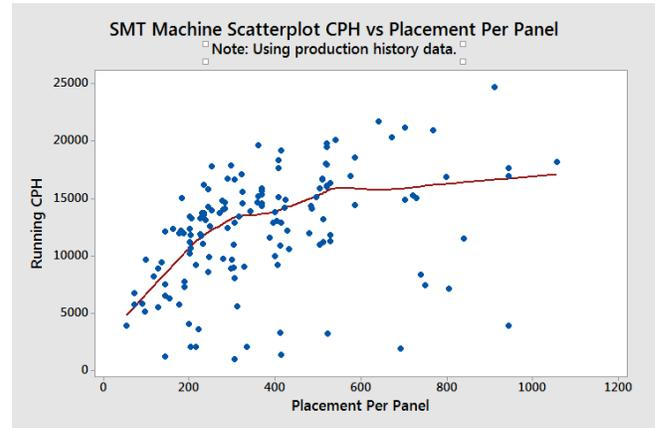
**Figure 1.** Scatter plot of CPH versus Placements per Panel from production data.
