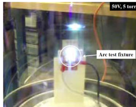
Figure 6. Example of a tin whisker initiating an electrical arc as shown in a CALCE experiment. (Courtesy of Center for Advanced Life Cycle Engineering [CALCE])
