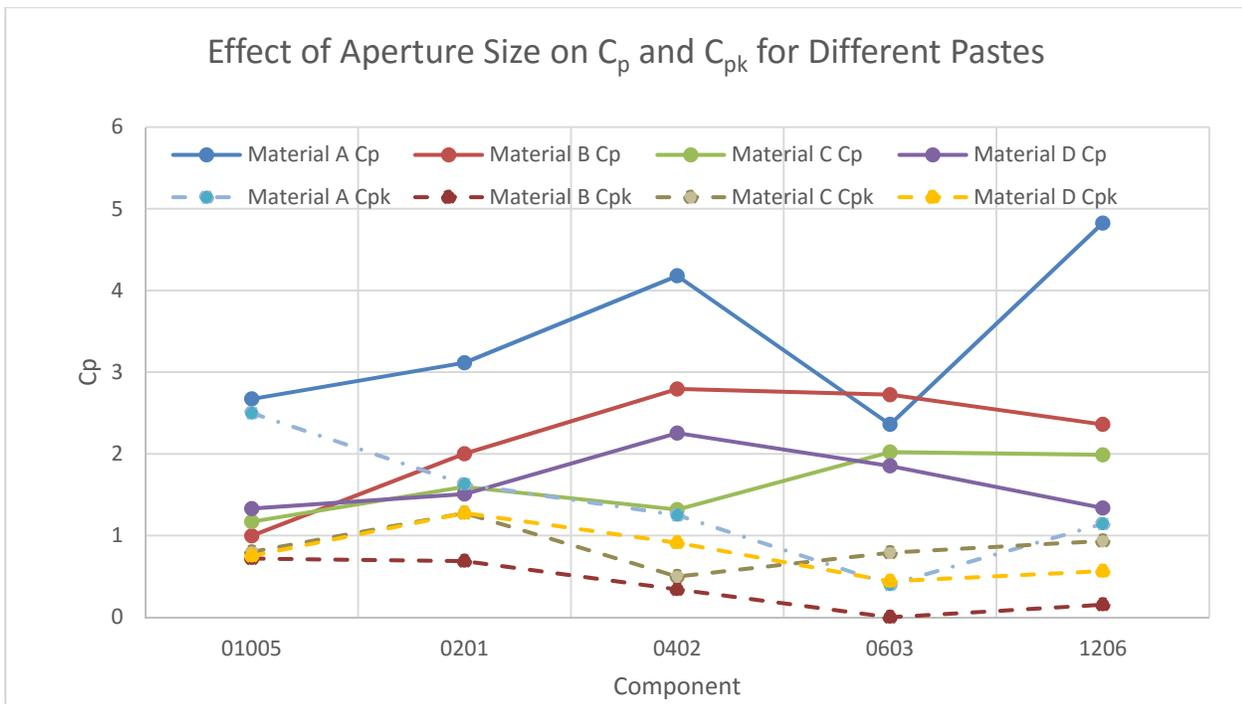
Figure 7: Effect of Aperture Size on  $C_p$  and  $C_{pk}$
