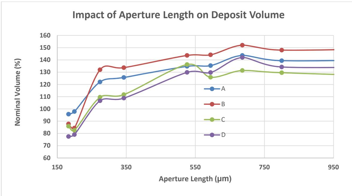
**Figure 5B:** Impact of Aperture Length on Deposit Volume
