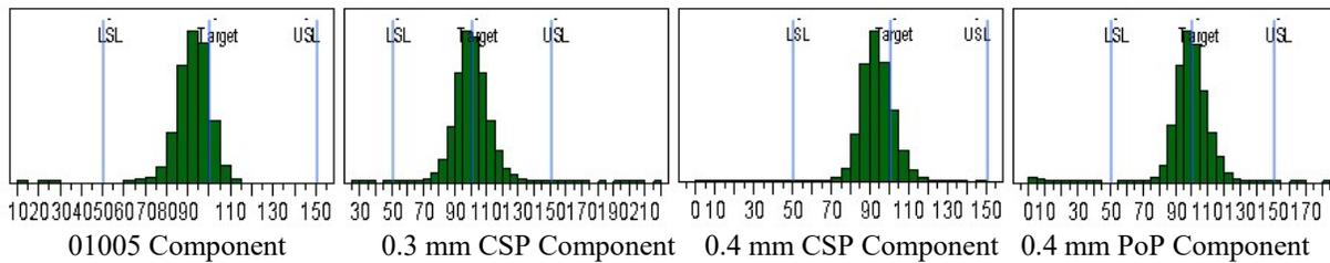
**Figure 12:** Effect of Eight Hour Abandon Time on Deposit Distributions for Apertures with Aspect Ratios below 0.66
