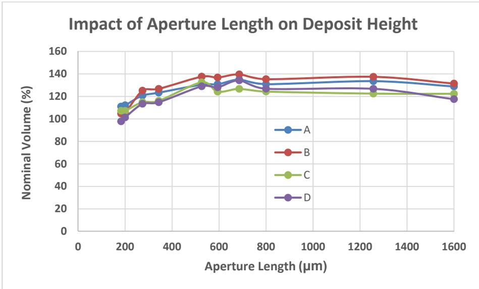
Figure 6A: Impact of Aperture Length on Deposit Height
