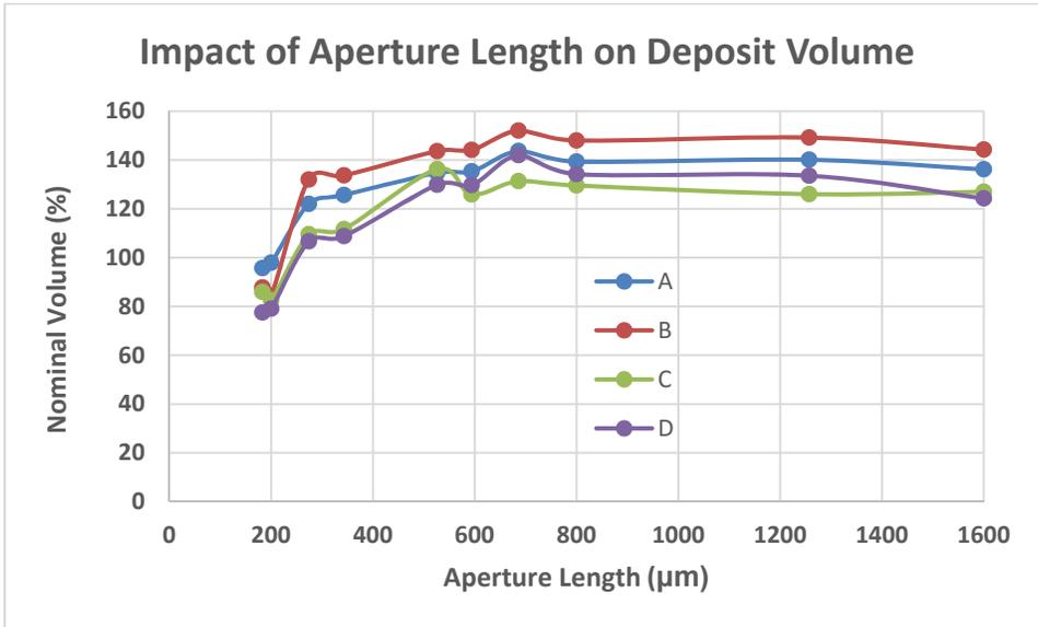
**Figure 5A:** Impact of Aperture Length on Deposit Volume
