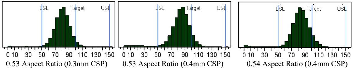
**Figure 8C:** Print Volumes Distributions for Low Aspect Ratio Square Apertures with Rounded Corners (Paste C)
