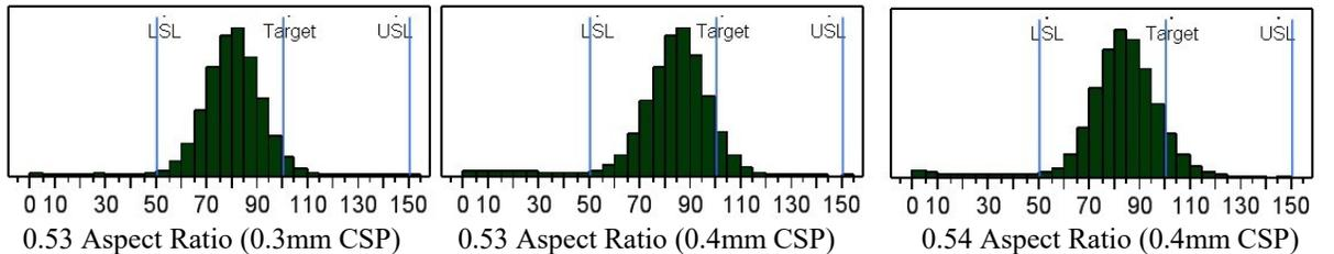
**Figure 8D:** Print Volumes Distributions for Low Aspect Ratio Square Apertures with Rounded Corners (Paste D)
