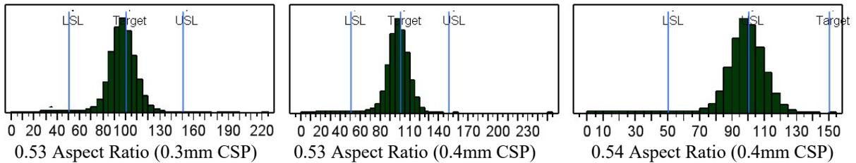
**Figure 8B:** Print Volumes Distributions for Low Aspect Ratio Square Apertures with Rounded Corners (Paste B)
