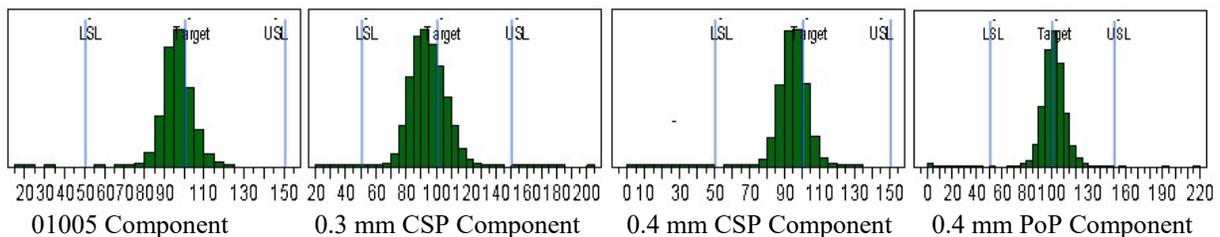
Figure 11: Effect of One Hour Abandon Time on Deposit Distributions for Apertures with Aspect Ratios below 0.66
