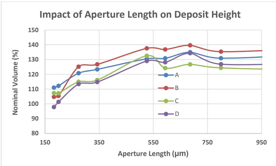
Figure 6B: Impact of Aperture Length on Deposit Height
