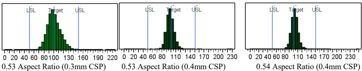
**Figure 8A:** Print Volumes Distributions for Low Aspect Ratio Square Apertures with Rounded Corners (Paste A)
