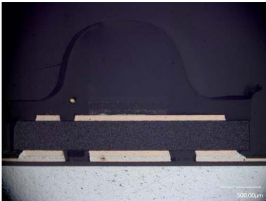
**Figure 9:** NC Paste # 2 with HR Pb-Free alloy on MCPCB-MP after 1000 cycles. Small cracks observed in solder joints on only one of the pads.
