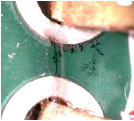
Figure 33: 1 st contact with the positive pad at 58 seconds
