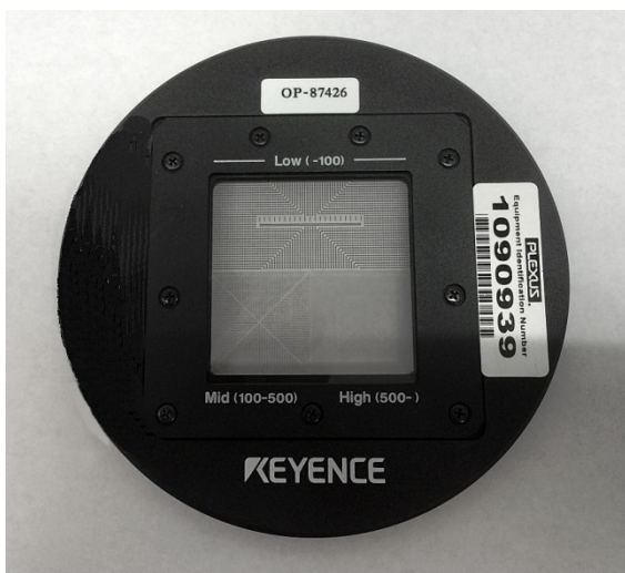
Figure 20: Glass slide with various size and space markings used to calibrate the measurements and insure accuracy.
