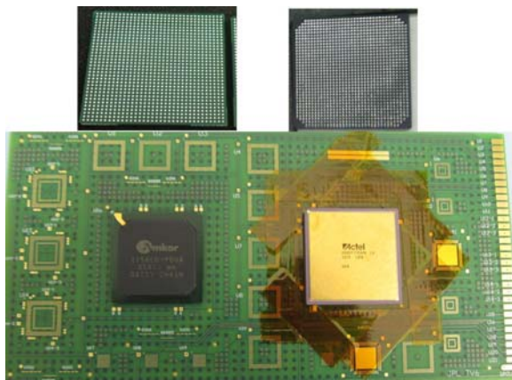
Figure 6. HDI PCB with plastic and ceramic high I/O packages LGA assembly. Both plastic 1156 I/O (top left) and ceramic 1272 I/O LGAs had solder paste added and reflowed before assembly.
