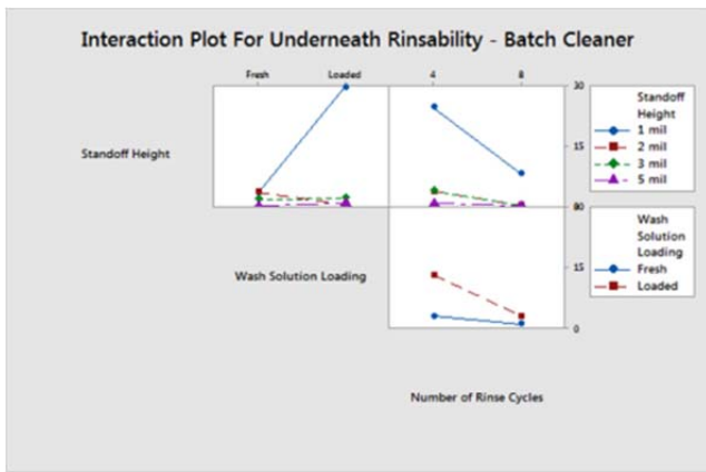
Figure 13. Batch Cleaner Analysis – Interaction Plot
