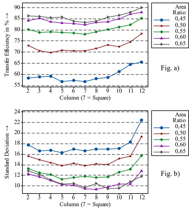
**Figure 5.** Influence of the aperture shape and the orientation for Solder Paste Type 4
