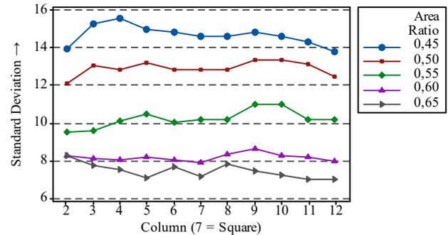
**Figure 7.** Influence of the aperture shape and the orientation for the 80  $\mu\text{m}$  stencil
