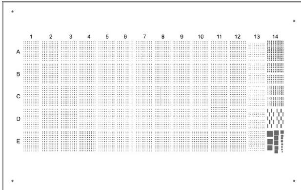
Figure 1. PCB and solder paste deposit layout
