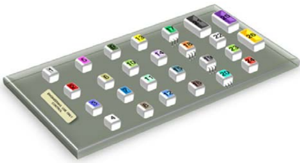
Figure 13. Illustrates the placement of various components with the different housing configurations that were epoxy attached to a common PCB as the test platform or vehicle.
