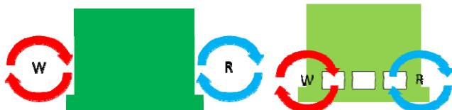
Figure 9. Components that are either hermitically sealed (L) or have ample vents or openings (R), then the washing / rinsing process will result in a “clean” component.
