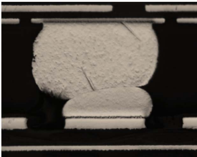
Figure 10. Typical HIP issue when using too long soak time and too high soak temperature. This issue could pass a functional test and end up as a field return.
