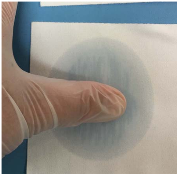
Figure 7. IPA glove application process with clean wipe soaked with IPA.
