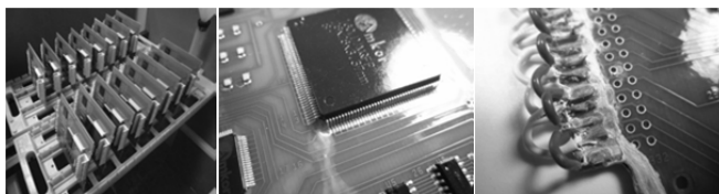
Figure 4: Boards for salt fog test as placed in the test chamber and after the completion of the test.
