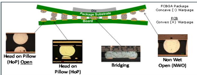
**Figure 2:** Description of defects that can be caused by dynamic warpage of FCBGA components and/or PCBs during the reflow soldering process
