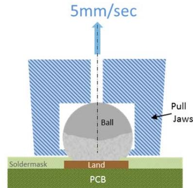
Figure 10: Schematic representation of Cold Ball Pull test condition
