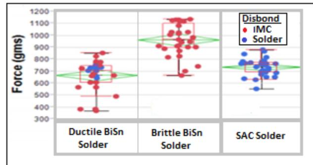
Figure 12: Cold Ball pull force and disband type for the SAC305/SAC305 and the SAC305/SnBi solder systems.
