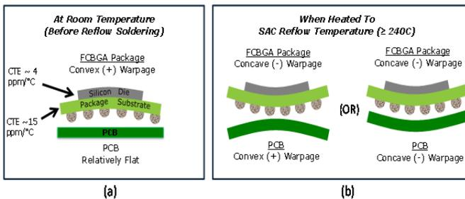
**Figure 1:** Typical warpage shapes of FCBGA packages and PCBs (a) at room temperature and (b) at SAC solder paste reflow temperatures
