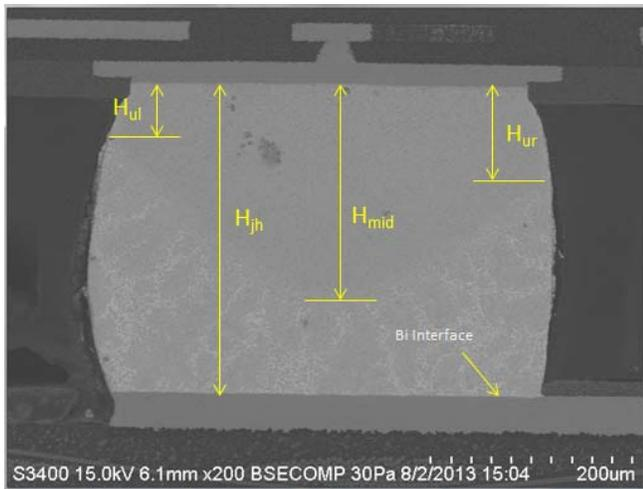
**Figure 4:** Cross section of a mixed SAC305 + SnBi solder joint indicating the height of diffusion of the Bi region into the joint
