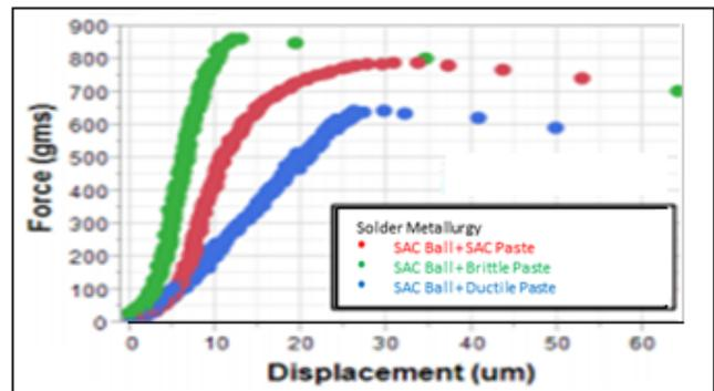
Figure 11: Force displacement curves comparing the SAC305/SAC305 system vs. SAC305/SnBi solder systems
