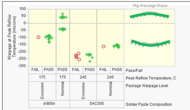
**Figure 7:** SMT yield and warpage comparison at 245C and 175C peak reflow temperatures
