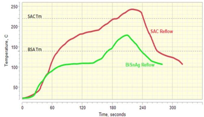
**Figure 8:** The Two Reflow Profiles used for the Power Use Savings Study
