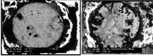
**Figure 13:** Images of the disband region after Cold Ball Pull joint fracture.
