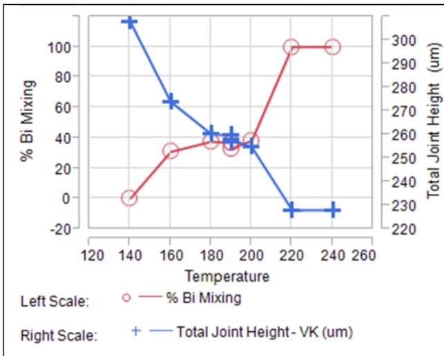
**Figure 5:** Bismuth mixing and solder joint collapse height as a function of peak reflow temperature
