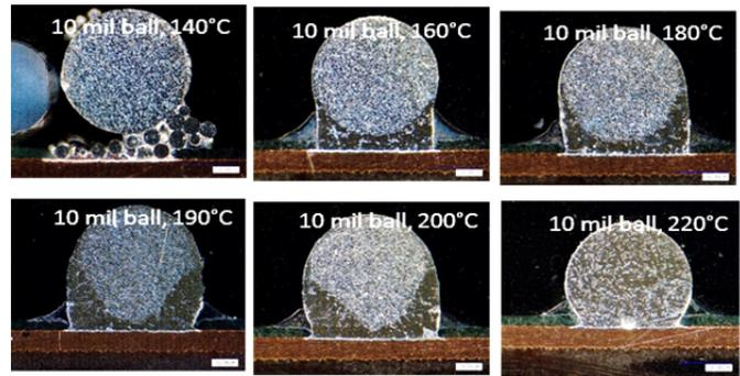
**Figure 6:** Cross section images of mixed SAC305 + SnBi solder paste solder joints after melting at the indicated temperatures.
