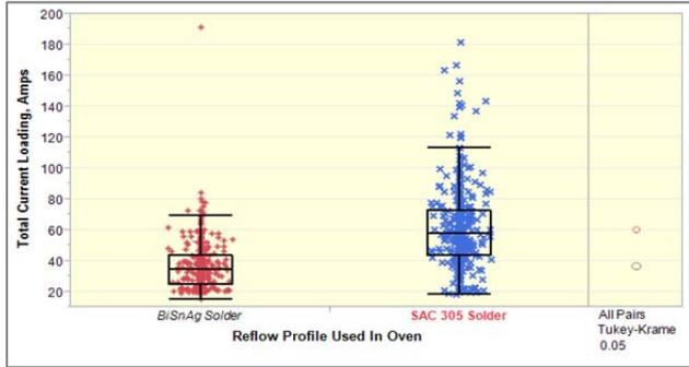
**Figure 9:** Comparison of Current Loading for a Reflow Oven when running a Low Temperature BSA soldering vs a standard SAC soldering reflow profiles
