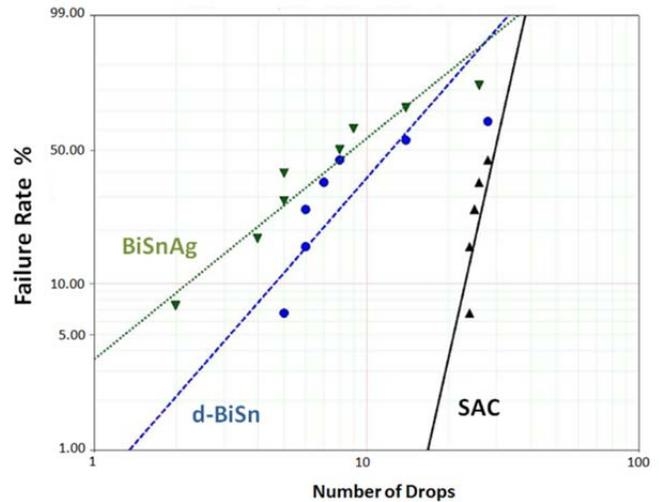
**Figure 14:** Weibull distribution of shock drop performance of the full SAC, SAC/BiSnAg and SAC/Ductile BiSn mixed alloy solder joints
