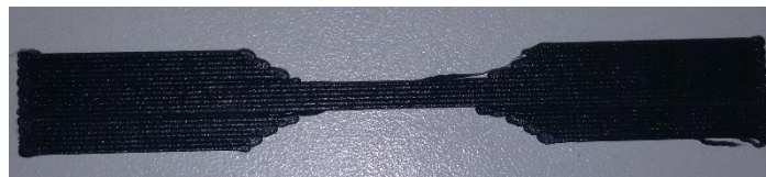
Figure 4: 0° Printed Tensile Specimen Using 0.4mm Nozzle
