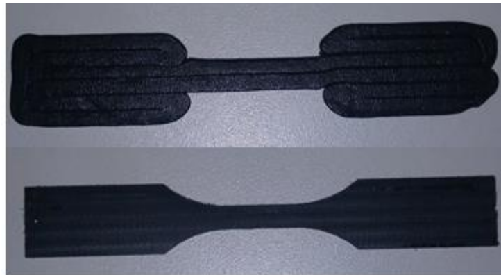
Figure 3: Spaghetti Printed Tensile Specimen Before and After Milling
