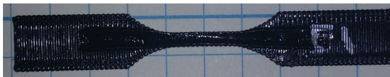
Figure 11: Laser "Reflowed" Tensile Part
