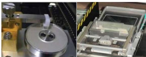
**Figure 8 – Dipping Station: Rotary Drum (left), linear squeegee (right)**
