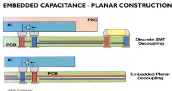
**Figure 4 – Buried Capacitance Inside PCB<sup>3</sup>**
