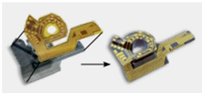
**Figure 12 – Molded Interconnect Device<sup>4</sup>**
