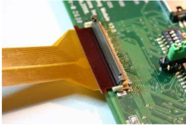
**Figure 2 – Board to FPC using connector**
