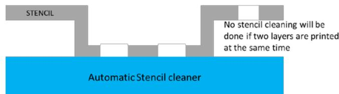
**Figure 10 – Automatic Stencil Cleaning Issue with One Pass**
