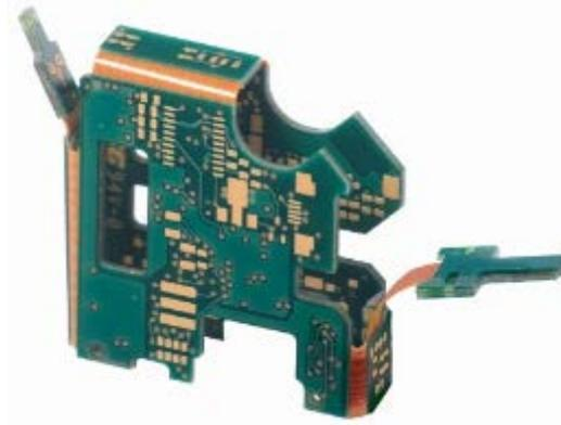
**Figure 3 – Example of a Rigid-Flex PCB<sup>2</sup>**
