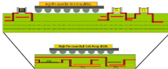
**Figure 5 – Embedded Passives inside PCB<sup>3</sup>**
