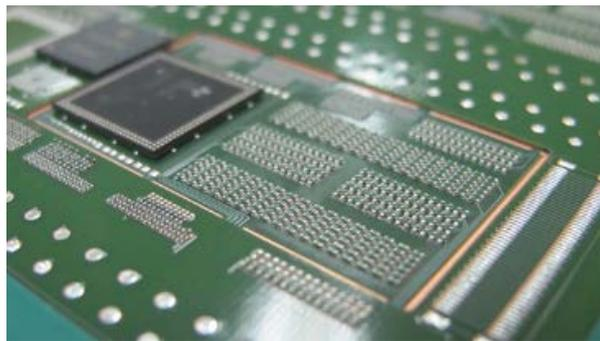
**Figure 9 – Cavity Assembly**
