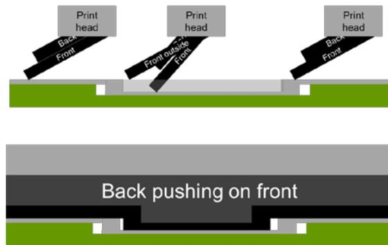
**Figure 11 – Slitted Squeegee with front and back blade**
